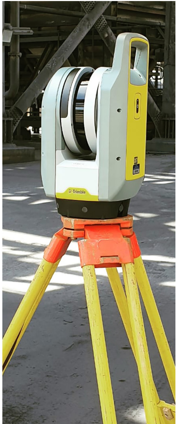
The Trimble X7 on site in Western Australia. The instrument's self-calibration and in-field registration significantly improved the SG crews' productivity.
