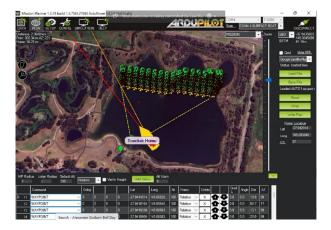
Due to time constraints, we also deployed a TriDrone RCV and manually navigated it through the shallow waters around the perimeter of the lake, covering the areas between where the automated mission run lines ended and the shoreline. Had the time not been of the essence, this "infill survey" could have been done by manually operating the HyDrone ASV following the completion of the automated survey.
