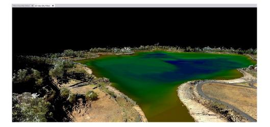
Trimble Business Center seamlessly integrated and consolidated GNSS observations, Optical Measurements, 3D Scans and Depth Soundings onto one project datum. From the combined data set, the edge of the lake was easily distinguished from the scan data and a surface was created to map the depths of the lake relative to the edge.
