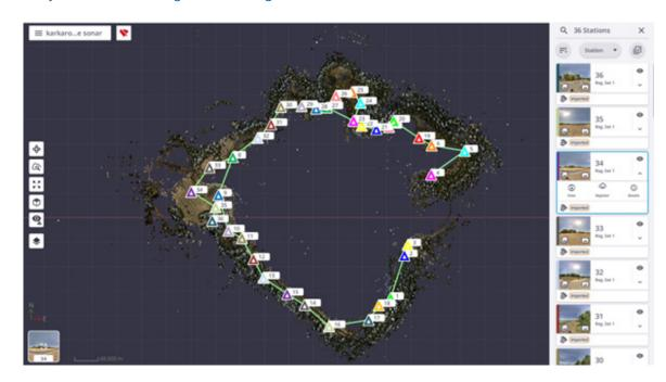
This provided real time insight into coverage from each scan station; identifying any gaps in the survey data and allowing the scanning team to infill where needed.
