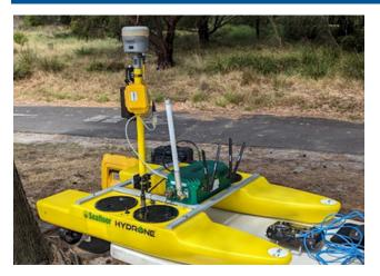
Positioning to the TriDrone was provided by a Trimble R780 GNSS receiver connected to Trimble VRSNow via 4G LTE, while the bathymetric survey was controlled by Trimble Access running on a Trimble TDC6 controller stowed away in the main pontoon payload bay.
